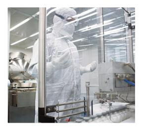
In aseptic manufacturing, eventual microorganisms are stopped before the process starts and the product doesn't exceed 20°C.
