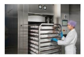
In the terminal sterilization process, the product must be treated with a high temperature autoclave process (at least 121°C) to kill eventual microorganisms inside. The dead bacteria will stay inside the cartridge or vial.
